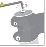
Tighten the headset bolt until pressure is felt using the allen key provided.
