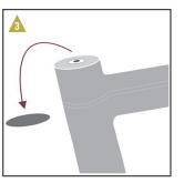
Sometimes there may be a plug in the top of the stem concealing the bolt. In this case pry the plug out carefully with a flat head screwdriver.
