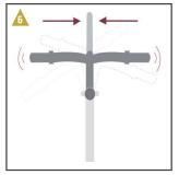
When the bolt is tight, hold the front wheel between your legs, and ensure that the handlebar won't twist easily under the pressure. If there is movement further stem bolt tightening is needed \*\*
