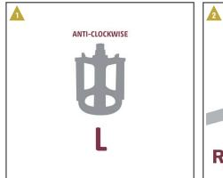
The right pedal will already be attached, but they can be identified by letters R and L stamped on the end of the axle or on the pedal body. R
