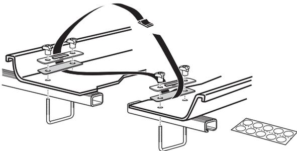
Fit the luggage straps underneath the 'U' bolt plates and rubber gaskets as shown. The metal plates must have the raised area facing upwards. Cover any unused mounting holes with the stickers provided.
