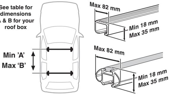
Ensure that the roof box you have purchased will fit your car and that your roof bars are of a suitable size to fit the fitting kit supplied with this roof box.
