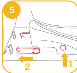
! Make sure that both ISOFIX connectors are securely attached to their ISOFIX anchor points. The colors of the indicators on both ISOFIX connectors should be completely green. 6 -1
