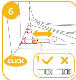
! If a tighter install or increased cabin space is required, then press the ISOFIX adjuster button 5 -1 and push to adjust. 6
