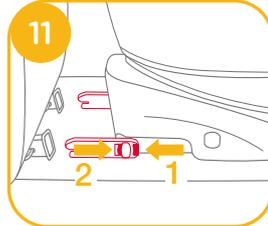
Then press and release the connectors from the vehicle's ISOFIX. **11**
