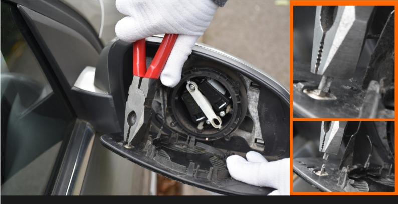
If mirror is heated, carefully remove the electrical connections, it maybe necessary to use a small pair of pliers.
