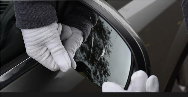
Carefully lift the glass from the mirror housing
