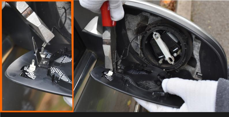
If mirror is heated replace the electrical connections onto the new mirror ensuring they are firmly in position
