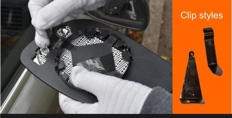
In certain circumstances you may have to install any clips provided onto the backing plate before fitting the mirror.
