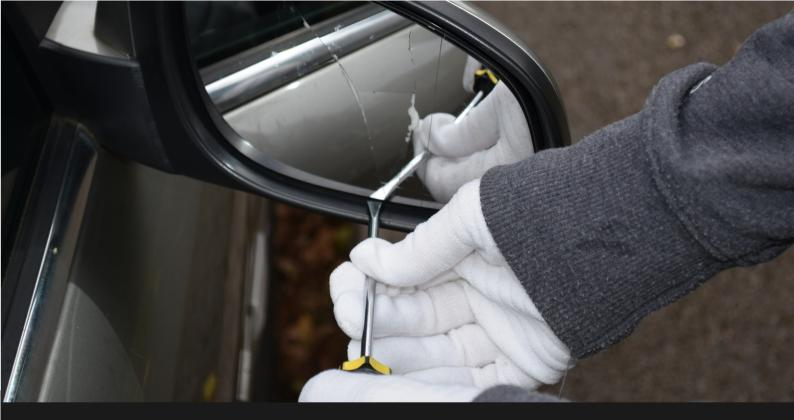
The original mirror can be removed by carefully placing a flat head screwdriver between the backing plate and mirror housing
