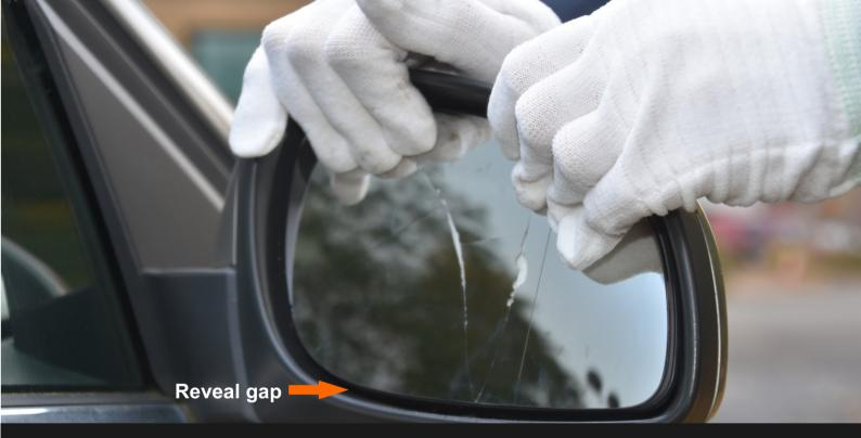
Apply pressure on the top part of the mirror pushing it inwards to reveal a gap at the bottom
