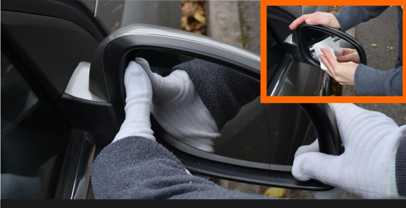
With the mirror securely in place straighten within the housing. Clean with a soft cloth and glass cleaner.
