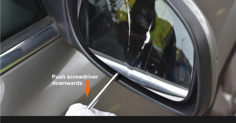
Carefully to avoid damaging the mirror housing push the screwdriver downwards to release the old glass
