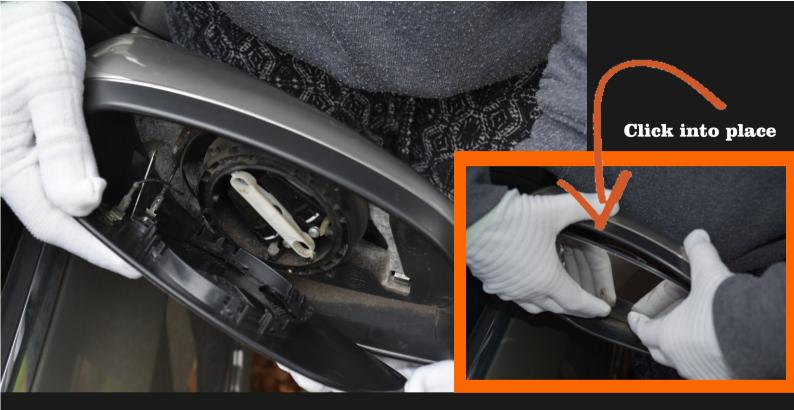
Line up the new mirror with the housing and apply pressure in the middle of the glass. As the mirror locates into place an audible click may be heard.
