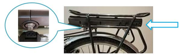
The battery must latch on with an audible click
