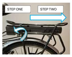
Unlock with the key & slide out the battery
