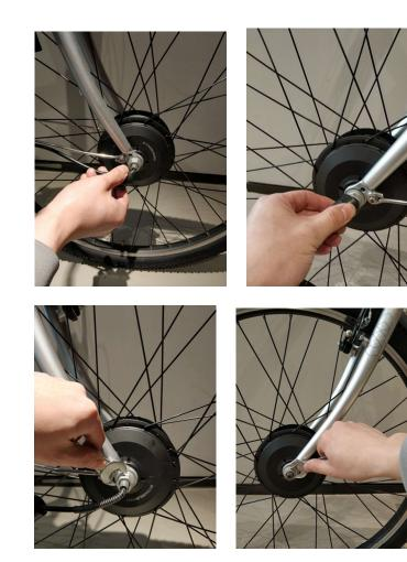
• Remove the rubber caps from both front wheel nuts & loosen the nuts (19 mm spanner). You may need to remove the nuts to release the wheel.
