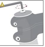
Tighten the headset bolt until pressure is felt using an allen key.
