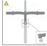
Line up the handlebar \* so that from above, it is at a 90° angle to the front wheel.
