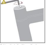
Tighten the bolt with an allen key, until resistance is felt. Reattach plug if needed.
