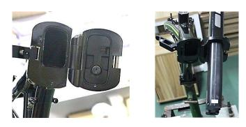
Unlock with the key & slide out the battery
