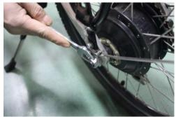
• Remove the rubber caps from both rear wheel nuts & loosen the nuts (19 mm spanner). You may need to remove the nuts to release the wheel.
