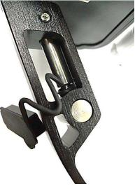
When the bike is folded always slide this protector over the two bladed contacts.
