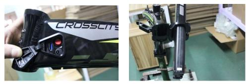
1. Push the battery into the end of the frame with the charging port on the left side
