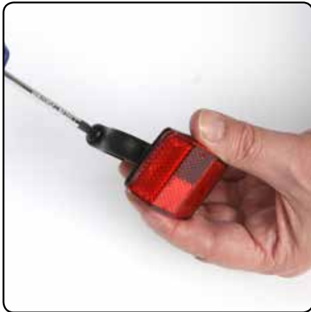
Take the rear (red) reflector and remove the screw as per the front reflector.
