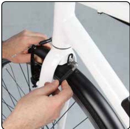
Insert a fixing screw and tighten using the Gtech tool provided.
