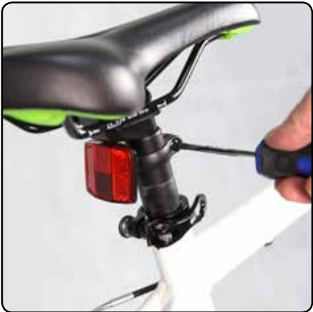
Clip the reflector to the seat post. Insert the screw and turn clockwise to secure the reflector in place.
