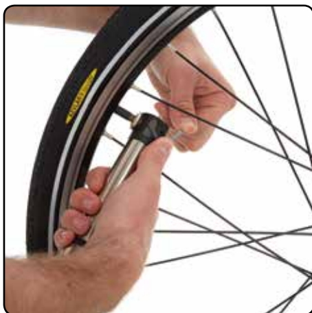
Lift the thumb lock lever into the locked position.
