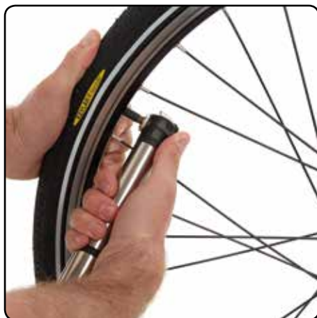
Press the pump nozzle onto the tyre valve stem as far as it will go.
