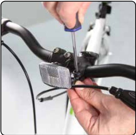
Clip the reflector to the handlebar. Locate the nut and insert the screw and turn clockwise to secure the reflector in place
