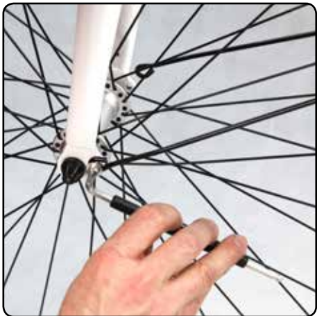
Position the stays against the fixing holes at the bottom of each side of the front forks. Insert a fixing screw at each side and tighten clockwise using the Gtech tool provided.
