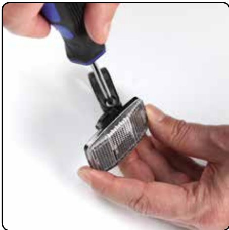
Use a Philips head screwdriver to turn the screw anti-clockwise to remove. Retain the nut.
