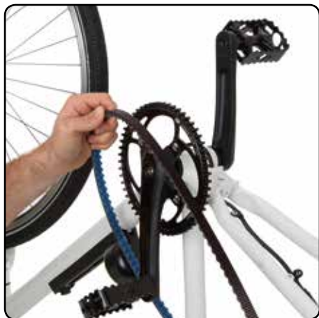
Take the belt off the pedal sprocket.
