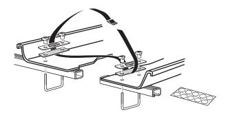
Fit the luggage straps underneath the 'U' bolt plates and rubber gaskets as shown. The metal plates must have the raised area facing upwards. Cover any unused mounting holes with the stickers provided.
