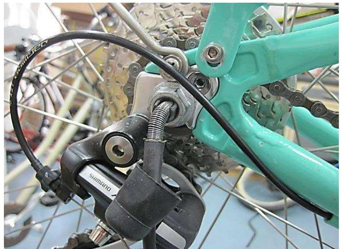
Having repaired the puncture, refit the wheel. Take care to ensure that the anti-rotation lugged washers on the axle are aligned with the drop outs.
