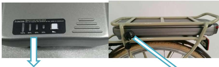
Battery level display and on/off 'Power' button
