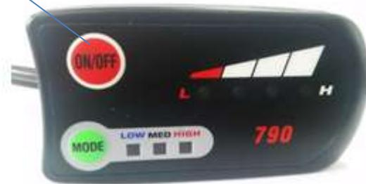
The handlebar display goes through a self-check routine, where all LEDs flash. The number of permanently lit red LEDs indicates the state of charge of the battery. The MODE defaults to 'LOW'.
