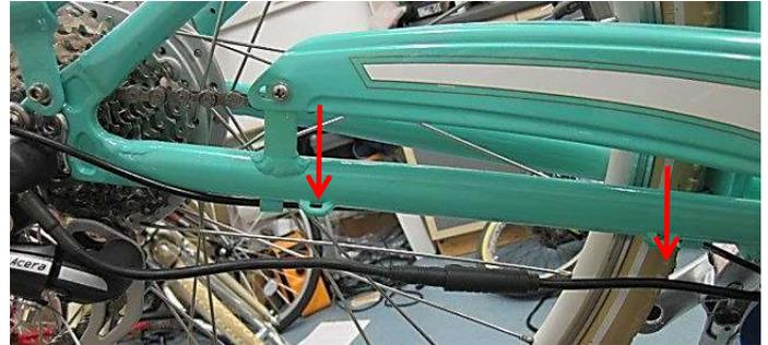
Unplug the two parts of the cable connector. You will need to 'wiggle' these parts to overcome the grip of the waterproof seal of this connector.
