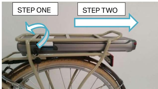
Unlock with the key & slide out the battery
