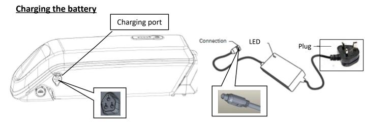
For safety this high energy density lithium-ion battery contains a sophisticated battery management system (BMS). The BMS ensures safe charging and discharge, continuously monitoring each of the cells in the battery individually. If the current drawn gets too high or the temperature of the battery is elevated, the BMS will shut the battery down for safety.
