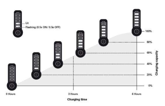
It is suggested to perform a complete discharge and recharge at every 3 months or after using 40 charging cycles in order to make the battery life longer.
