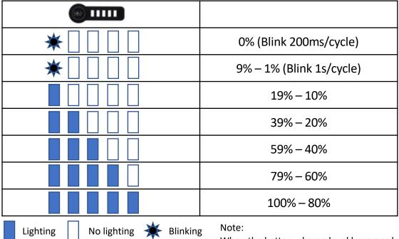
When the battery charge level becomes less than 5%. The output power will be reduced.
