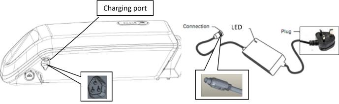
For safety this high energy density lithium-ion battery contains a sophisticated battery management system (BMS). The BMS ensures safe charging and discharge, continuously monitoring each of the cells in the battery individually. If the current drawn gets too high or the temperature of the battery is elevated, the BMS will shut the battery down for safety.
