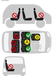
The suitable location for installation in the car is shown on the left:
